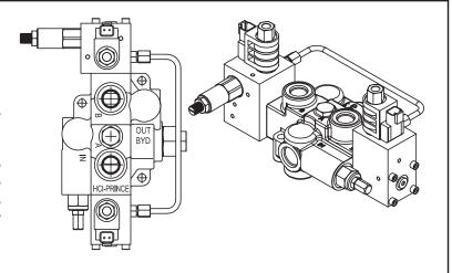
The RD5000 proportional operators are typically controlled with a thumb or handle control and a PWM control module. Prince offers a small thumb control joystick (671300076) and a larger handle control joystick (671300077). A PWM control module (671300107) that can be used in conjunction with these joysticks is also offered by Prince. See page V52 for details.
