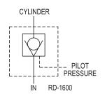
The PRINCE valve model RD-1600 is a pilot operated check valve. This valve blocks oil from flowing from the cylinder port to the valve port until sufficient pressure is applied to the pilot port. Oil can free flow from the valve port to the cylinder port. The valve has a two stage poppet allowing smooth chatter free operation.
